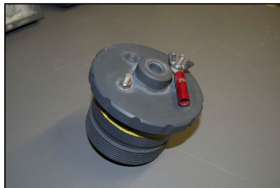
Figure 4.3: Connecting point of chloride conductivity cell
